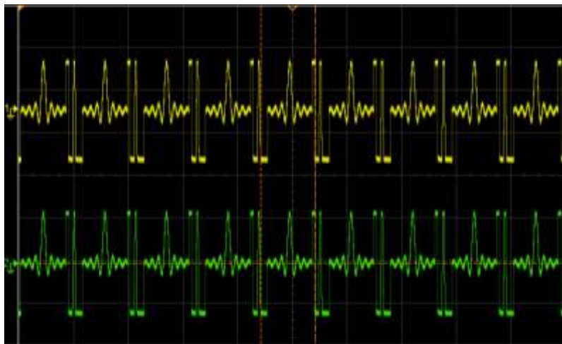
The two WX2184C after synchronization completed.
